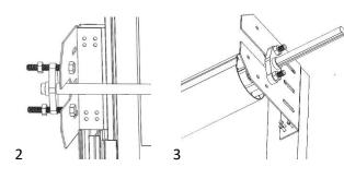
Install the drum and bearings.
