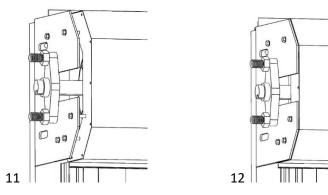
Finally, mount the top cover so that it fits flush between the two flags. If there is a gap between the top cover and the flags, it means that the installation has been made incorrectly.
