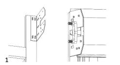
Attach the plate to the bottom zero, at a distance that will fit the top cover, and to the bottom zero point of the plate.
