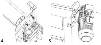
Place the motor on the shaft and connect the plate.
