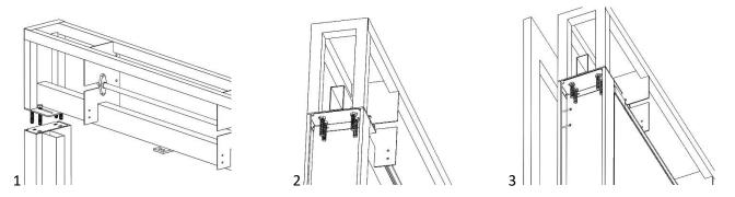
Complete the frame installation by joining the upper assembly and the uprights. Fix the mechanical assembly to the mounting surface.
