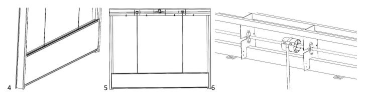
Put the tarpaulin between the uprights and lay it on the ground. Screw the tarpaulin suspension belts tightly to the upper drum.
