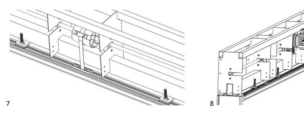
Roll the belts upwards by starting the engine in a controlled manner. Tighten the hanger screws and tighten the nuts.
