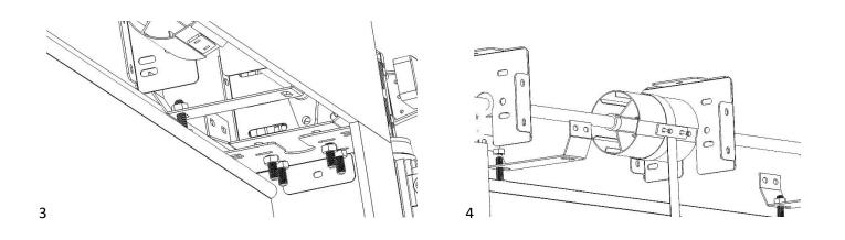
AFTER INSTALLATION OF THE MECHANICAL SECTION IS FINISHED, INSTALL THE TRAP HANGER SCREWS. SCREW THE TAPE BELTS TO THE DRUMS TOGETHER WITH THE PLATE.
