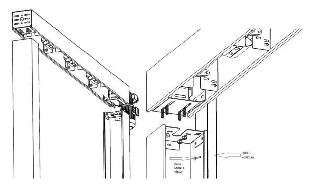
1 -2 CONNECT THE VERTICAL STRUCTURES AND UPPER ASSEMBLY GROUP SO THAT THE CORNERS ARE COMBINED AND COME ACROSS. FIX THE VERTICAL STRUCTURES AND TOP GROUP ASSEMBLY TO THE BACK SURFACE.
